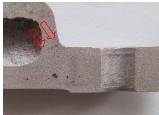
Figure 6. Crack in the inner area of the connection of the base to the wall.
